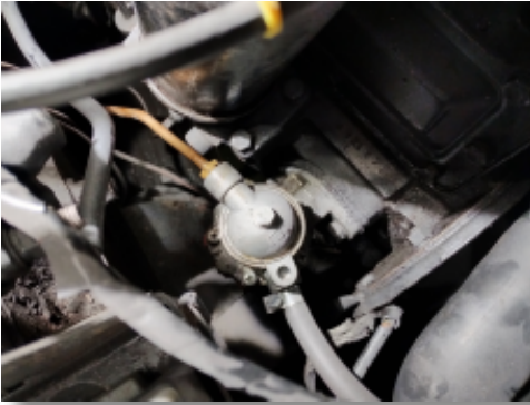
Above: the annoying modern "pattern" pump, unable to see if there's any dirt in the system and also without a mechanical priming lever. Above right: a very satisfying operational glass bowl pump complete with working priming lever.
