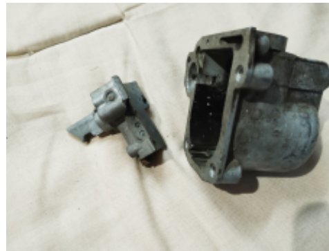
There are more jets in the small block in the side of the float chamber. The accelerator pump works on a piston with another jet below it. This particular piston is wedged in place and therefore this float chamber is now unusable.
