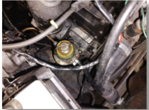
Above: the annoying modern "pattern" pump, unable to see if there's any dirt in the system and also without a mechanical priming lever. Above right: a very satisfying operational glass bowl pump complete with working priming lever.
