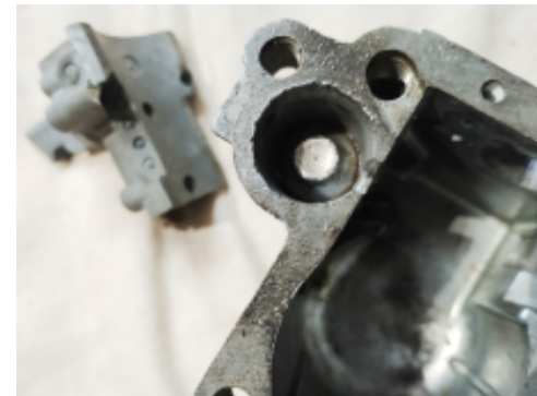
There are more jets in the small block in the side of the float chamber. The accelerator pump works on a piston with another jet below it. This particular piston is wedged in place and therefore this float chamber is now unusable.
