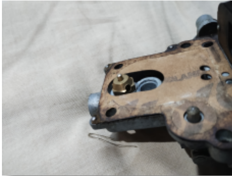
Above: test the inlet valve closes properly by blowing into the inlet when the piston is held closed. The mixture screw should be replaced with the same number of turns it took to remove. This is ideally tuned with the help of a Gunson Color Tune kit.
